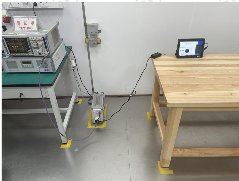
Conducted emission Test Setup
