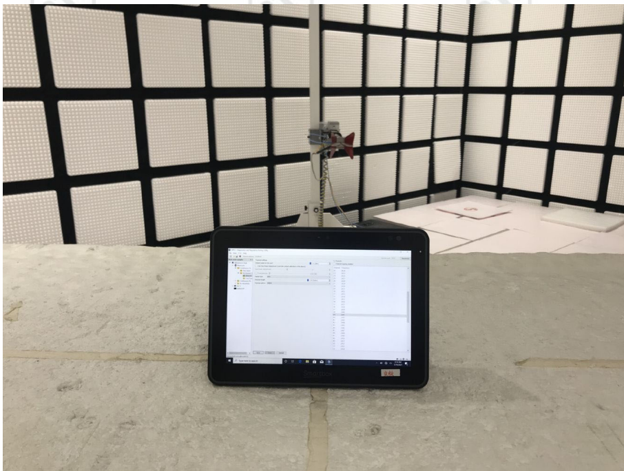
Radiated spurious emission Test Setup-2(Above 1GHz)
