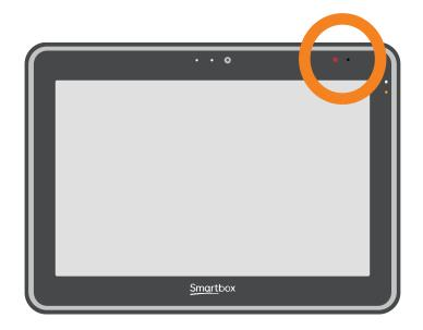
The IR receiver is used to learn controls from IR remotes.
