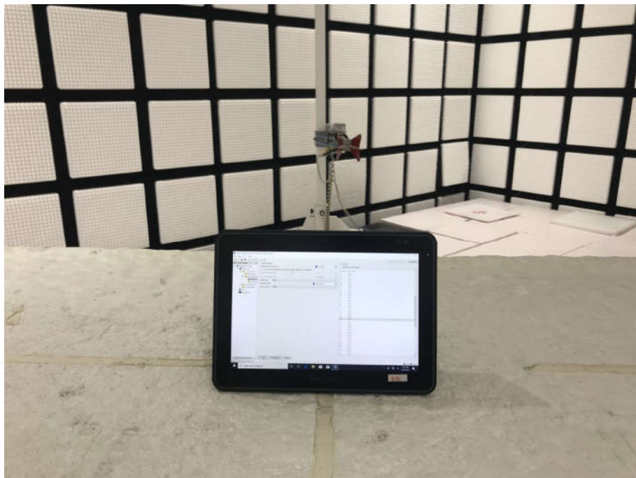
Radiated spurious emission Test Setup-2(Above 1GHz)
