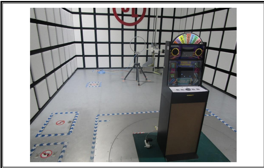
RADIATED RF MEASUREMENT SETUP (Below 30 MHz)
