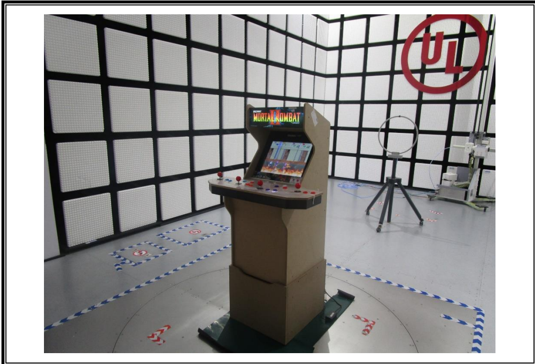
RADIATED RF MEASUREMENT SETUP (Below 30MHz)
