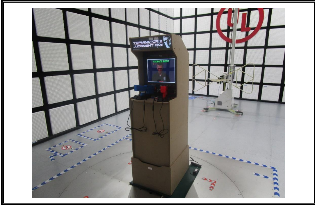
RADIATED RF MEASUREMENT SETUP (30MHz ~ 1 GHz)
