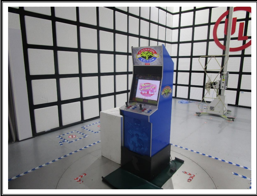
RADIATED RF MEASUREMENT SETUP (30MHz ~ 1 GHz)
