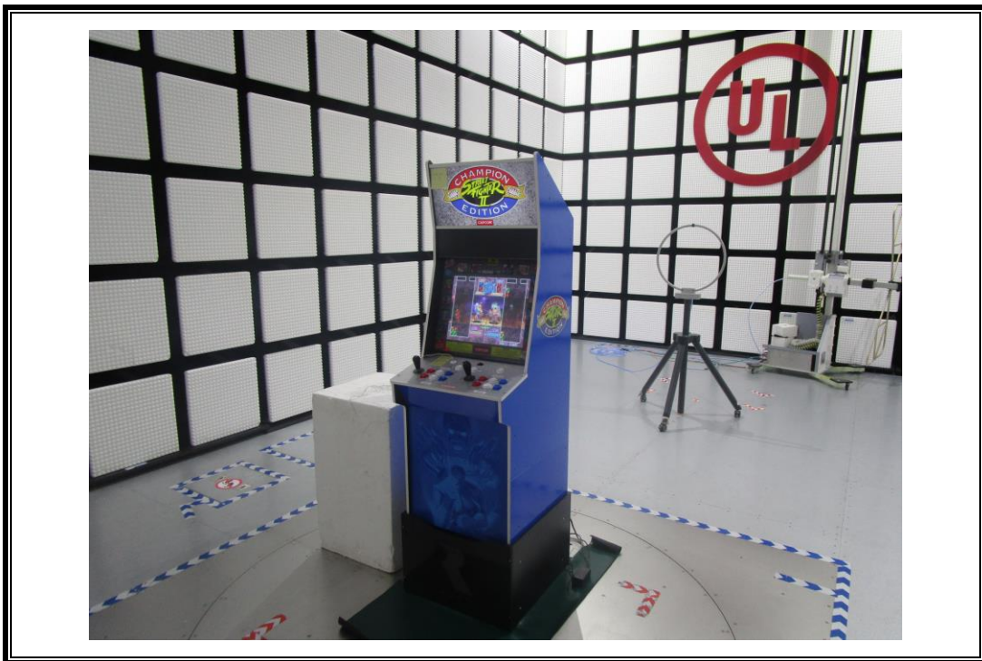
RADIATED RF MEASUREMENT SETUP (Below 30MHz)
