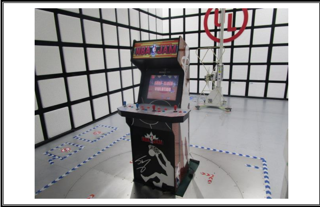
RADIATED RF MEASUREMENT SETUP (30 MHz ~ 1 GHz)
