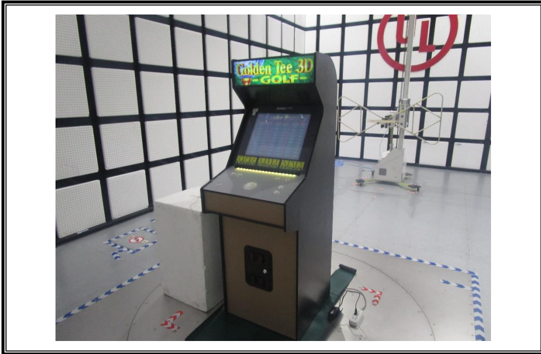
RADIATED RF MEASUREMENT SETUP (30MHz ~ 1 GHz)
