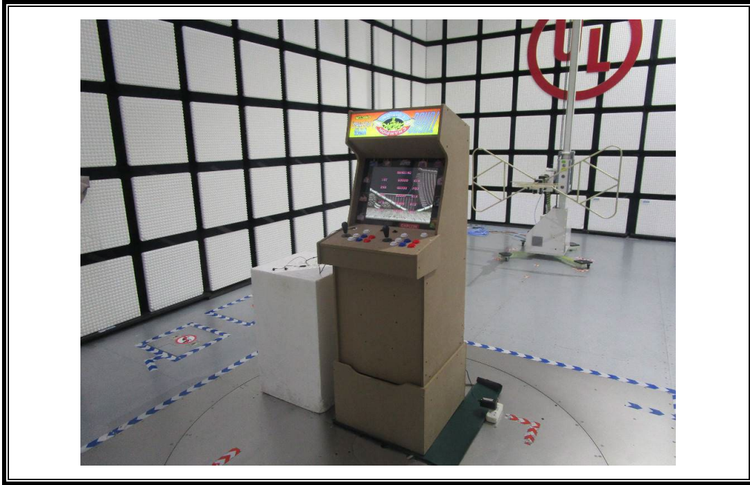
RADIATED RF MEASUREMENT SETUP (30 MHz ~ 1 GHz)
