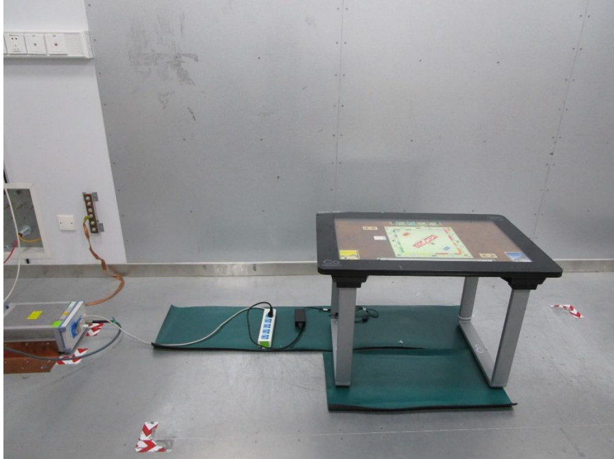
POWERLINE CONDUCTED EMISSIONS MEASUREMENT SETUP
