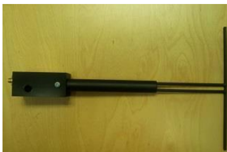
Figure 1 – MVG COMOSAR Validation Dipole
