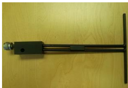
Figure 1 – MVG COMOSAR Validation Dipole
