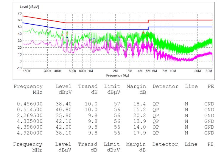
Note: 1. Result Level = Read Level +LISN Factor + Pulse Limiter Factor + Cable loss.
