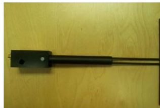
Figure 1 – MVG COMOSAR Validation Dipole
