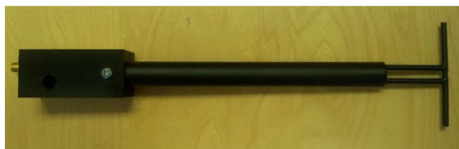
Figure 1 – MVG COMOSAR Validation Dipole
