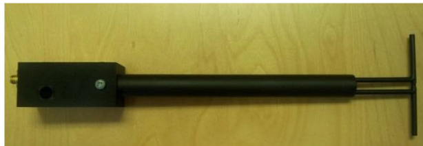
Figure 1 – MVG COMOSAR Validation Dipole
