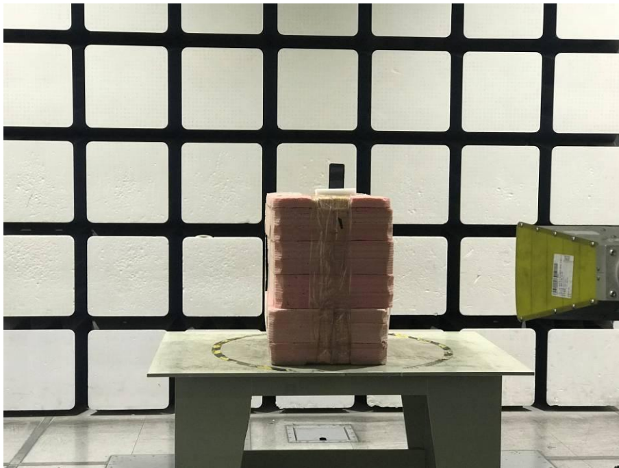
Radiated Emissions View (Above 1 GHz)
