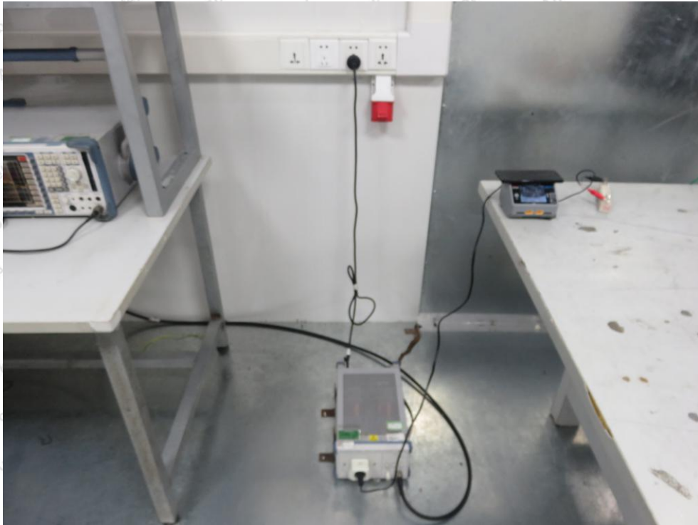
Photo of Conducted Emission Measurement
