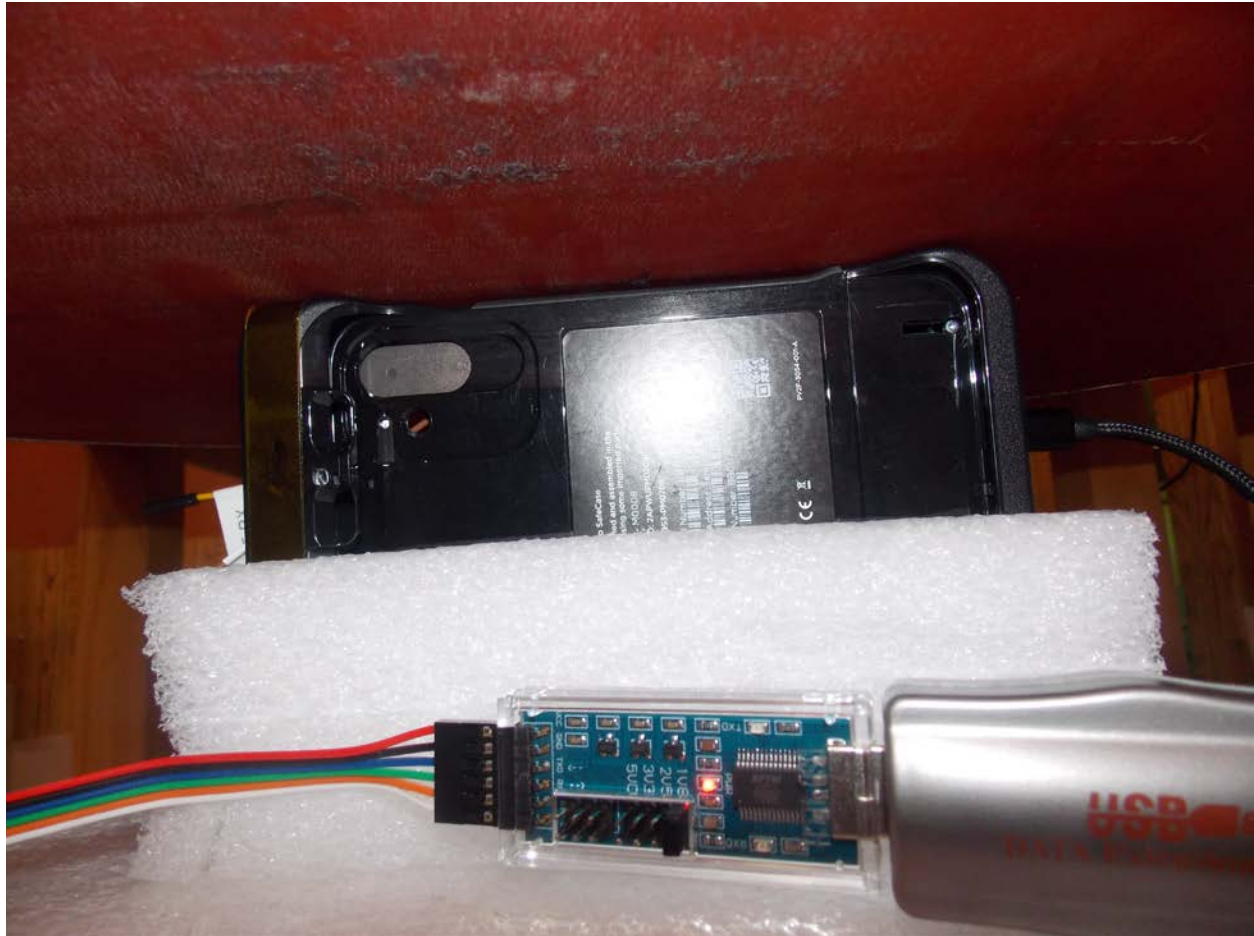
Body Right Configuration 5 mm Gap
