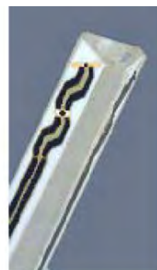
Figure 2.3 Probe Thick-Film Technique
