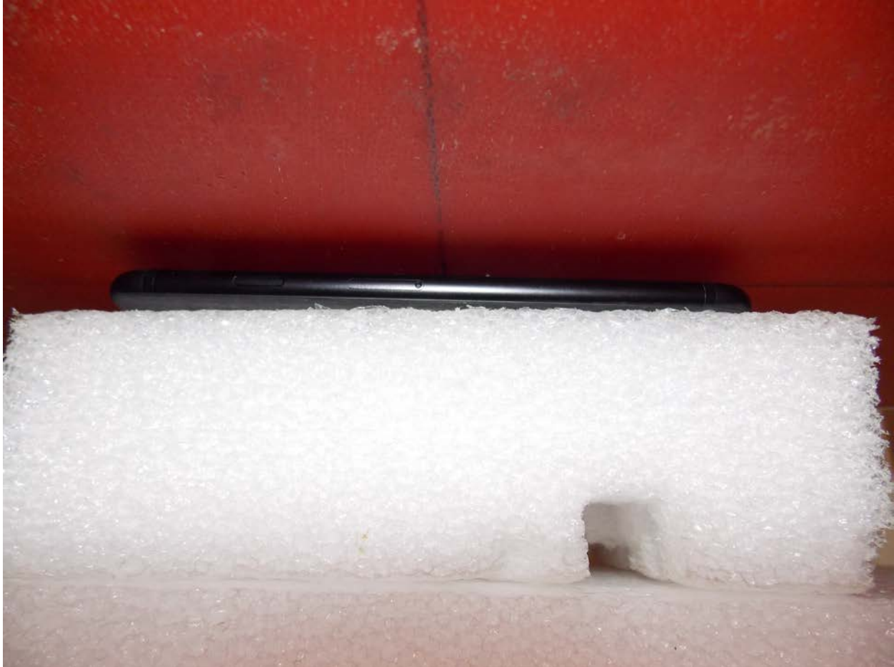
Body Back Configuration No Case 5 mm Gap
