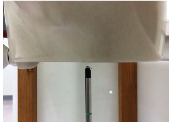
Fig.6 EUT Bottom side to flat phantom
