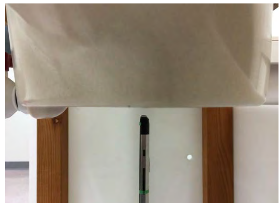
Fig.8 EUT Left side to flat phantom
