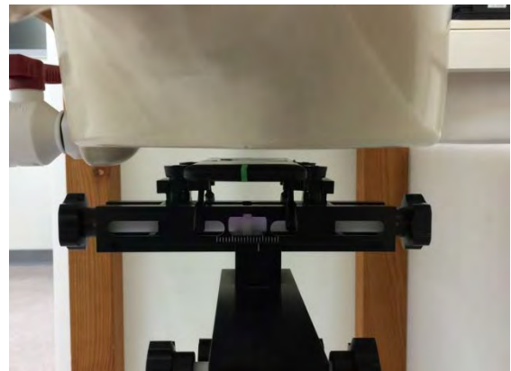
Fig.4 EUT Back side to flat phantom
