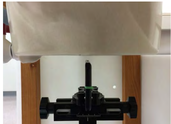
Fig.7 EUT Right side to flat phantom
