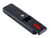
2. Insert the fresh battery, and please ensure the batteries are put in a correct direction. Do not install the batteries in the reverse direction as this could cause the batteries to leak corrosive liquids, generate heat or explode.
