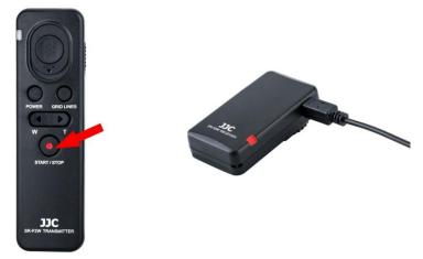
2. To stop recording, press the video recording button again. The status lamp lights in green.
