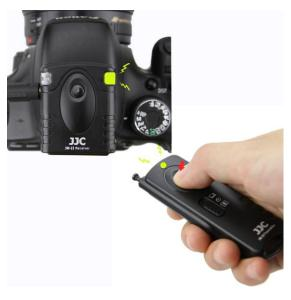
2. Then fully press the shutter button, and the camera will take a picture after 5 seconds count down. You will get a delay shot photo.
