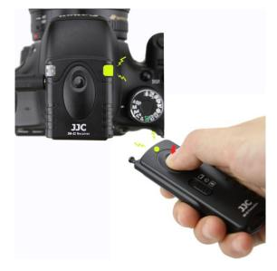
2. Then fully press while holding the shutter button of transmitter until the transmitter LED light OFF, and the receiver will now lock the shutter for BULB.
