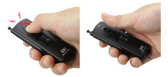
3. To release the shutter lock, press the shutter button of the transmitter again, and the receiver will unlock the shutter. Then you will get plenty of pictures.
