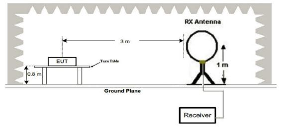
(2) Radiated Emission Test-Up Frequency 30MHz~1GHz
