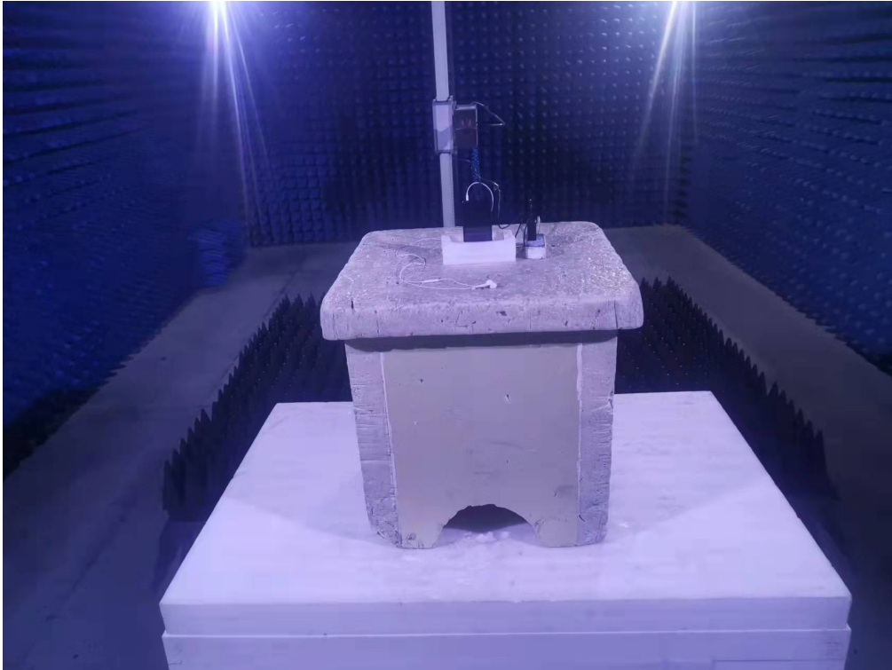
Photo of Radiated Emission Measurement (Above 1G)
