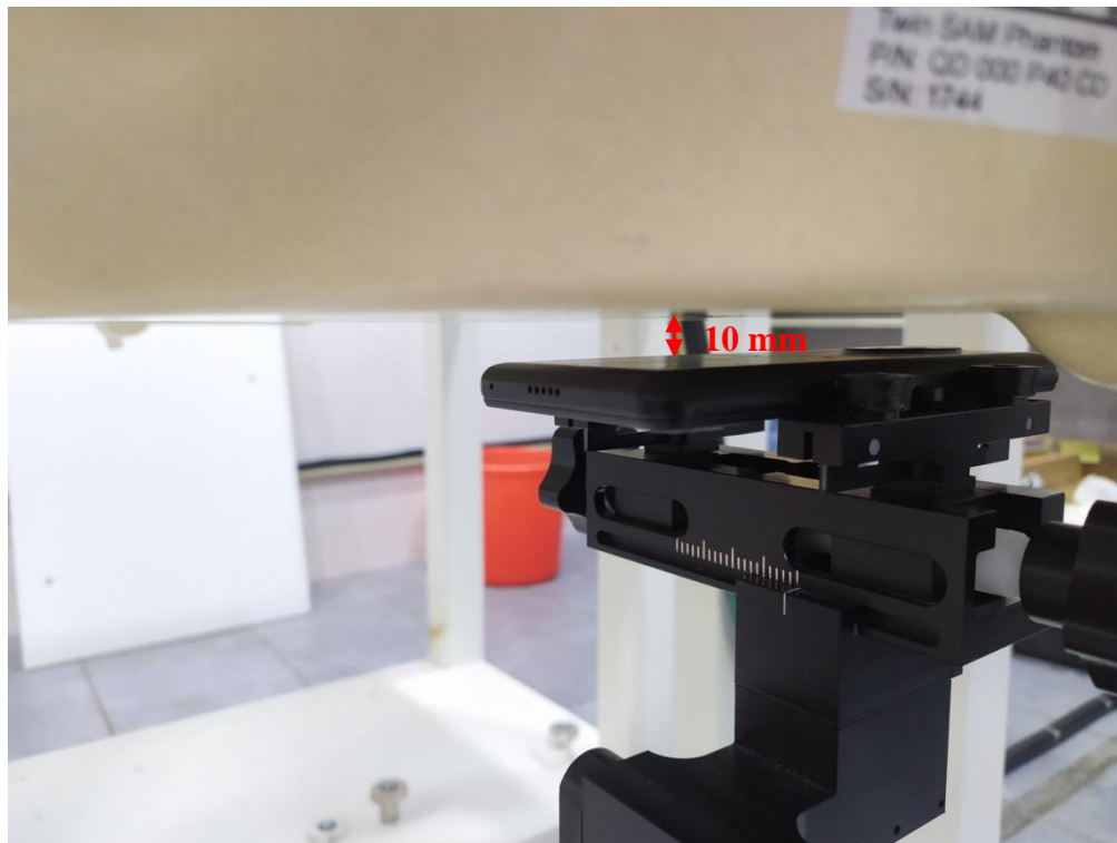
Body (Worn) Back Setup Photo (10mm)
