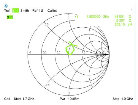
Calibrated return loss: -26.66dB; Measurement return loss: -27.3 dB(within 20%)
