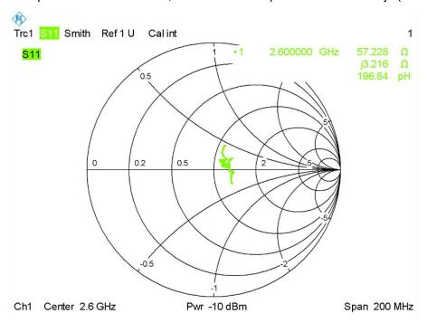
Calibrated return loss: -24.86dB; Measurement return loss: -23.1 dB(within 20%)
