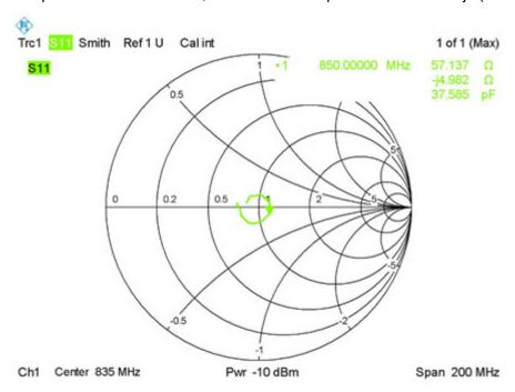
Calibrated return loss: -24.51dB; Measurement return loss: -22.89 dB(within 20%)
