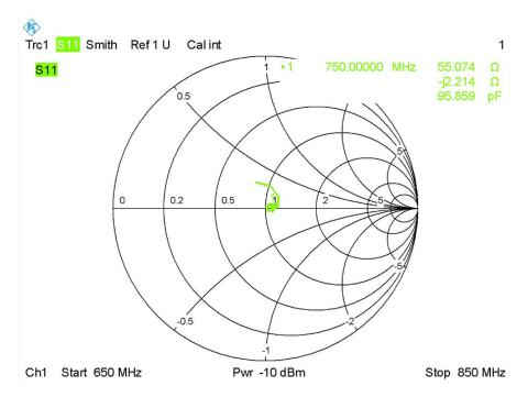
Calibrated return loss: -25.20dB; Measurement return loss: -23.05 dB(within 20%)
