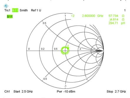
Calibrated return loss: -24.86dB; Measurement return loss: -23.18 dB(within 20%)
