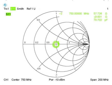
Calibrated return loss: -25.20dB; Measurement return loss: -24.41 dB(within 20%)
