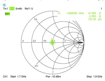
Calibrated return loss: -26.66dB; Measurement return loss: -28.54 dB(within 20%)
