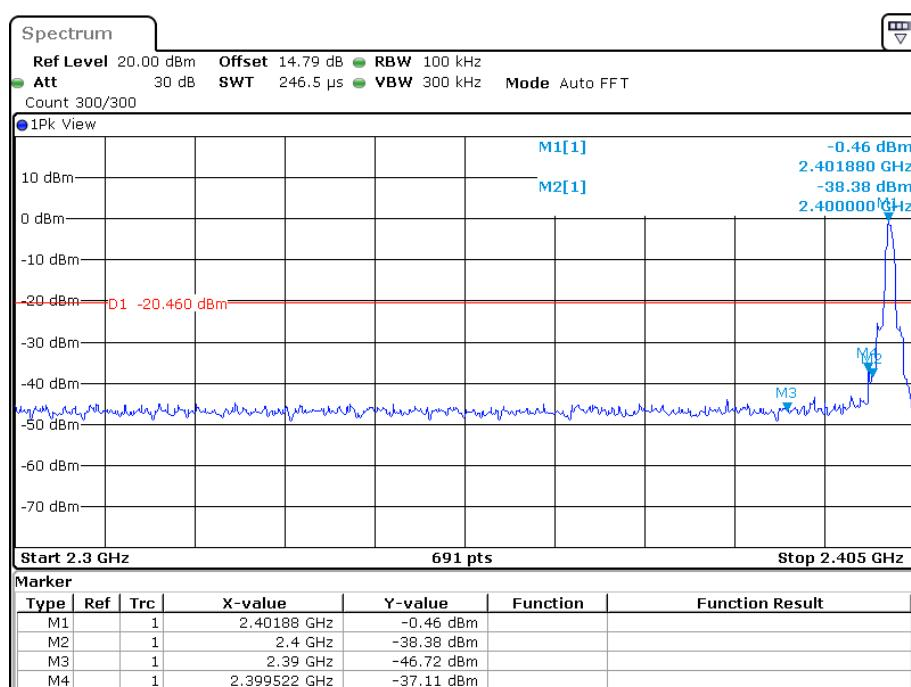
**EDR ( $\pi/4$ -DQPSK): Band Edge-Right Side****Hopping**
