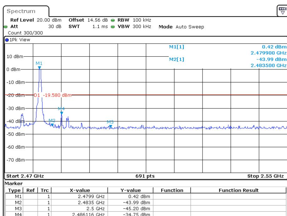
**EDR ( $\pi/4$ -DQPSK): Band Edge-Left Side****Hopping**
