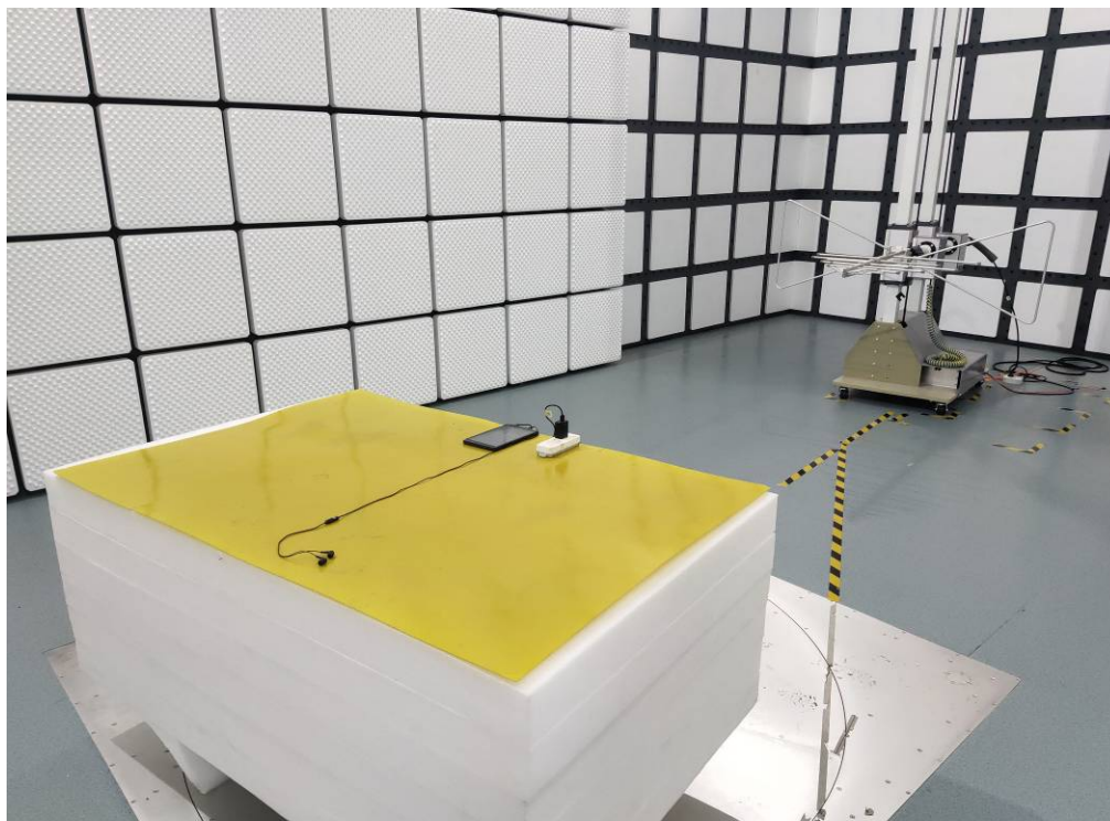
Photo of Radiated Emission Measurement (Below 1G)
