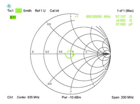
Calibrated return loss: -24.51dB; Measurement return loss: -22.89 dB(within 20%)
