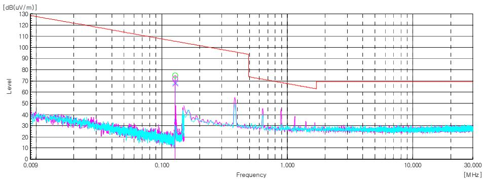
**- 7.5 W Charging Mode (Less than 50 % of Battery)**
