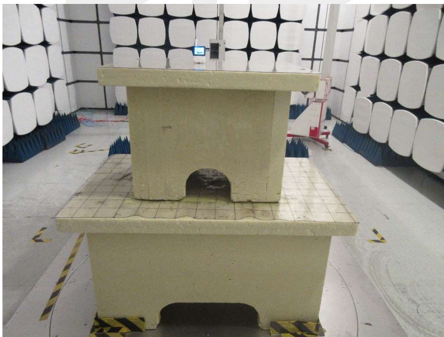
Radiated SPURIOUS EMISSION SET-UP PHOTOS, 1GHz ~ 18GHz
