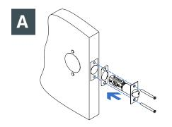
Slide latch into edge bore of the door. Check that the faceplate does not project outside door, but it should also not be installed sunk.
