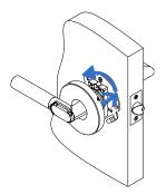
Attach the covers of both the door handles by placing it on the holder and turning it.
