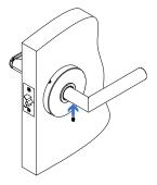
Insert the locking screw from the bottom of the mechanical door handle and tighten it.
