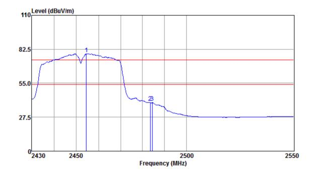
Mode:a; Polarization:Horizontal; Modulation:n; bandwidth:40MHz; Channel:High
