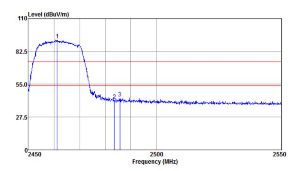
Mode:a; Polarization:Horizontal; Modulation:n; bandwidth:20MHz; Channel:High
