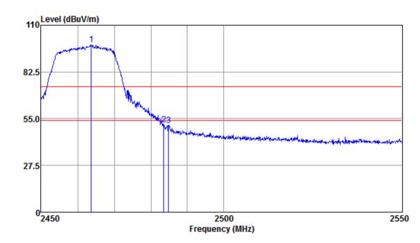
Mode:a; Polarization:Vertical; Modulation:g; bandwidth:20MHz; Channel:High
