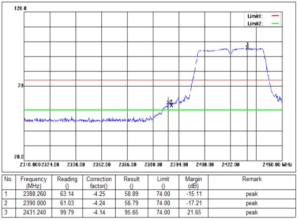
Mode:a; Polarization:Vertical; Modulation:n; bandwidth:40MHz; Channel:Low
