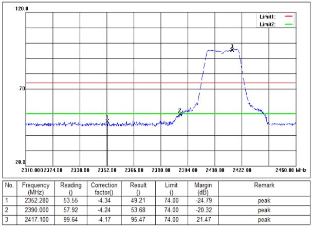
Mode:a; Polarization:Horizontal; Modulation:n; bandwidth:20MHz; Channel:Low
