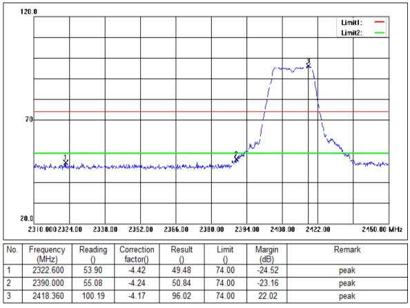
Mode:a; Polarization:Horizontal; Modulation:g; bandwidth:20MHz; Channel:Low
