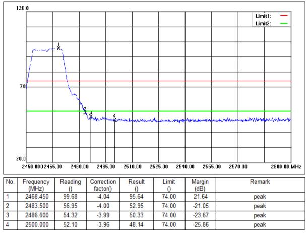
Mode:a; Polarization:Horizontal; Modulation:n; bandwidth:20MHz; Channel:High
