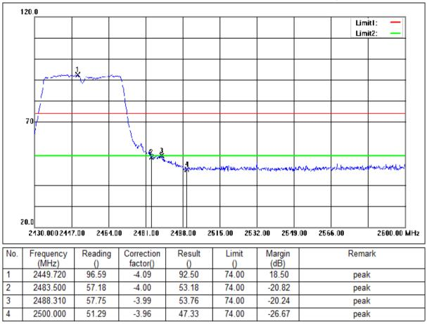
Mode:a; Polarization:Horizontal; Modulation:n; bandwidth:40MHz; Channel:High
