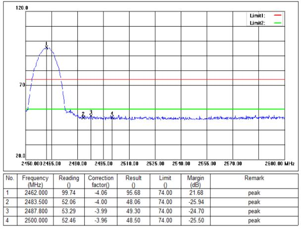
Mode:a; Polarization:Horizontal; Modulation:b; bandwidth:20MHz; Channel:High
