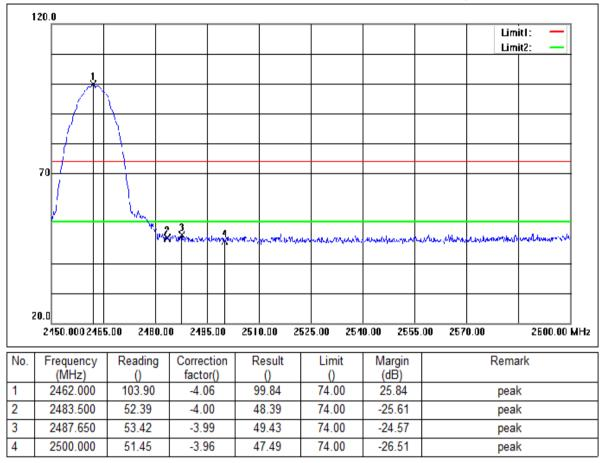
Mode:a; Polarization:Vertical; Modulation:b; bandwidth:20MHz; Channel:High
