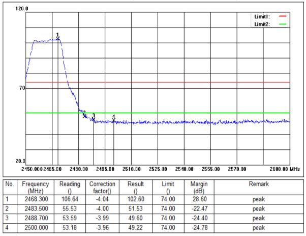
Mode:a; Polarization:Vertical; Modulation:g; bandwidth:20MHz; Channel:High
