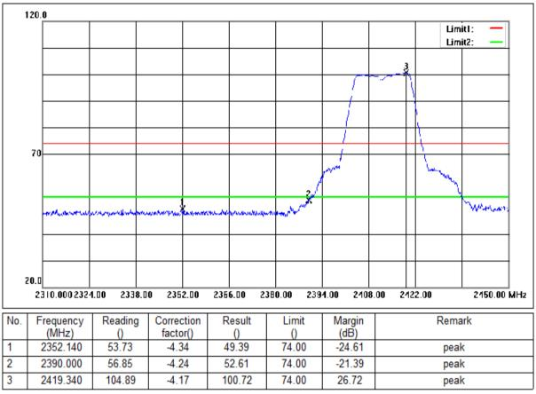
Mode:a; Polarization:Vertical; Modulation:n; bandwidth:20MHz; Channel:Low
