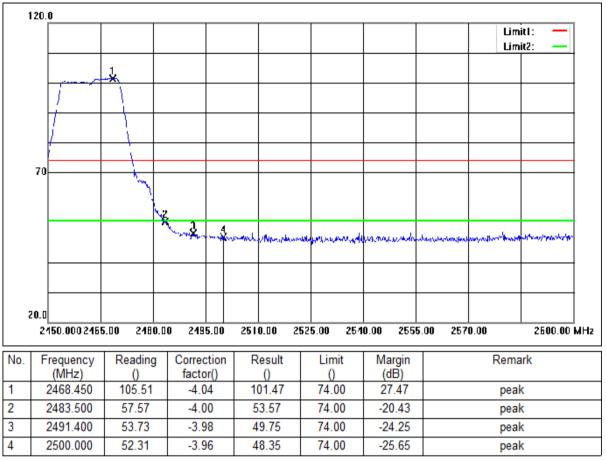
Mode:a; Polarization:Vertical; Modulation:n; bandwidth:20MHz; Channel:High
