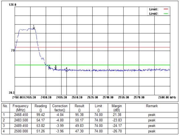
Mode:a; Polarization:Horizontal; Modulation:g; bandwidth:20MHz; Channel:High
