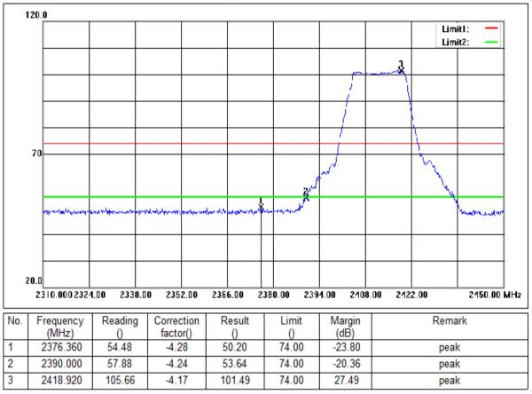
Mode:a; Polarization:Vertical; Modulation:g; bandwidth:20MHz; Channel:Low
