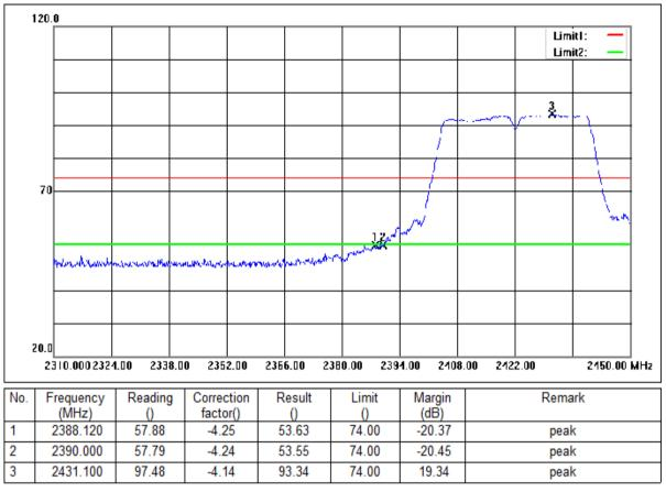
Mode:a; Polarization:Horizontal; Modulation:n; bandwidth:40MHz; Channel:Low
