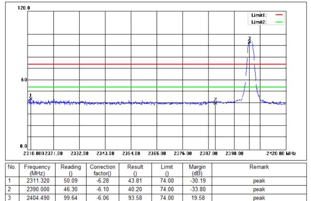
Mode:a; Polarization:Vertical; Modulation:O-QPSK; Channel:Low
