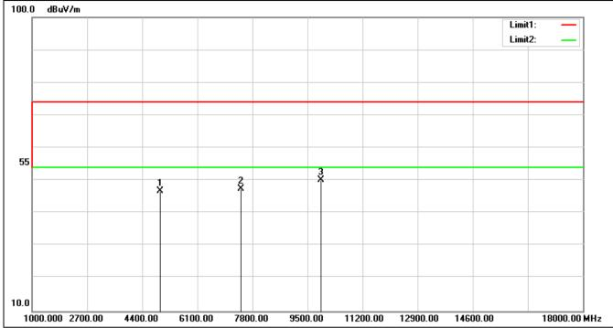
Mode:a; Polarization:Vertical; Modulation:O-QPSK; Channel:High
