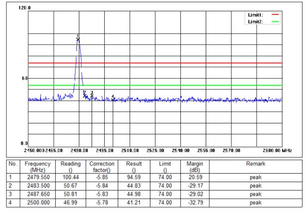
Mode:a; Polarization:Horizontal; Modulation:O-QPSK; Channel:High
