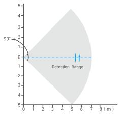
Fig. 2 Top view of the detection range
