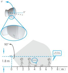
Fig. 1 Side view of the detection range
