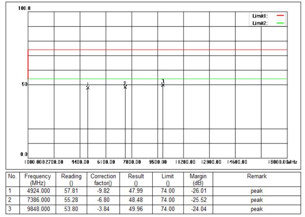
Mode:a; Polarization:Horizontal; Modulation:g; bandwidth:20MHz; Channel:High
