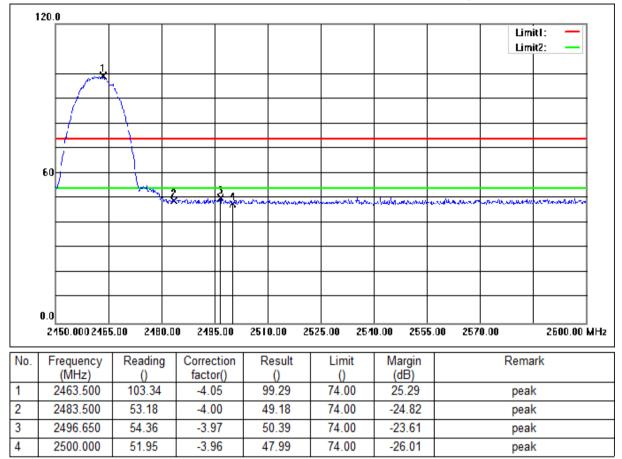
Mode:a; Polarization:Vertical; Modulation:b; bandwidth:20MHz; Channel:High
