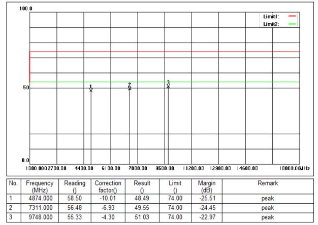
Mode:a; Polarization:Vertical; Modulation:b; bandwidth:20MHz; Channel:middle
