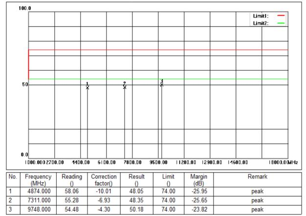
Mode:a; Polarization:Vertical; Modulation:g; bandwidth:20MHz; Channel:middle
