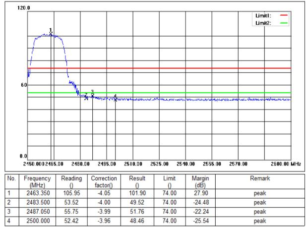
Mode:a; Polarization:Horizontal; Modulation:g; bandwidth:20MHz; Channel:High
