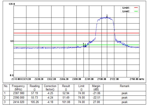
Mode:a; Polarization:Vertical; Modulation:n; bandwidth:20MHz; Channel:Low
