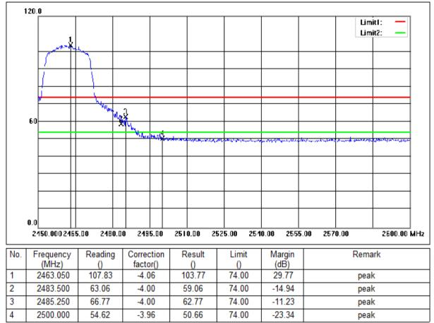
Mode:a; Polarization:Horizontal; Modulation:n; bandwidth:20MHz; Channel:High
