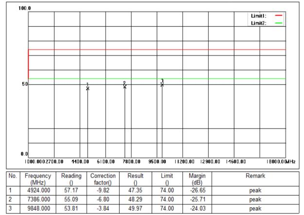
Mode:a; Polarization:Vertical; Modulation:b; bandwidth:20MHz; Channel:High
