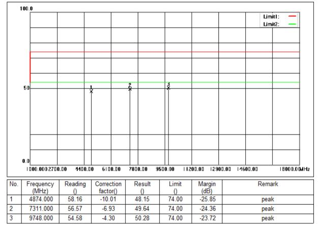
Mode:a; Polarization:Horizontal; Modulation:b; bandwidth:20MHz; Channel:middle
