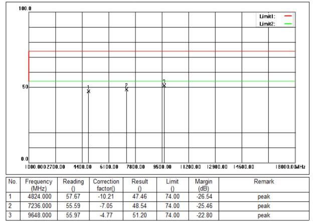
Mode:a; Polarization:Vertical; Modulation:g; bandwidth:20MHz; Channel:Low
