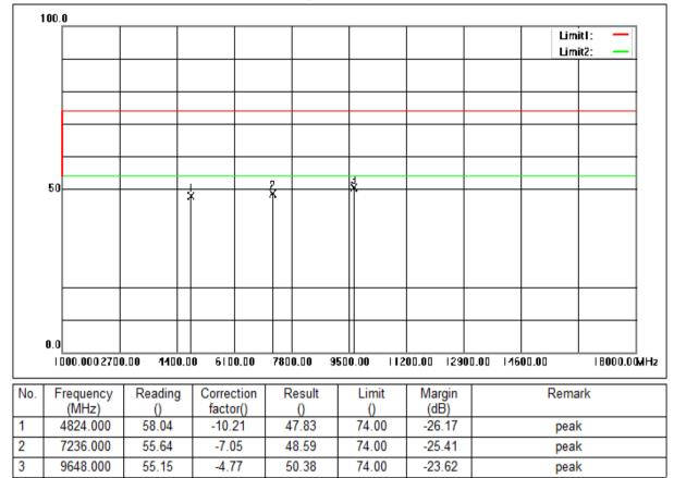
Mode:a; Polarization:Horizontal; Modulation:g; bandwidth:20MHz; Channel:Low
