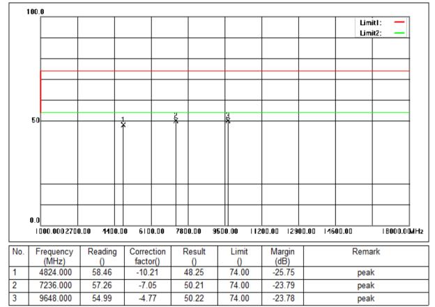
Mode:a; Polarization:Vertical; Modulation:b; bandwidth:20MHz; Channel:Low
