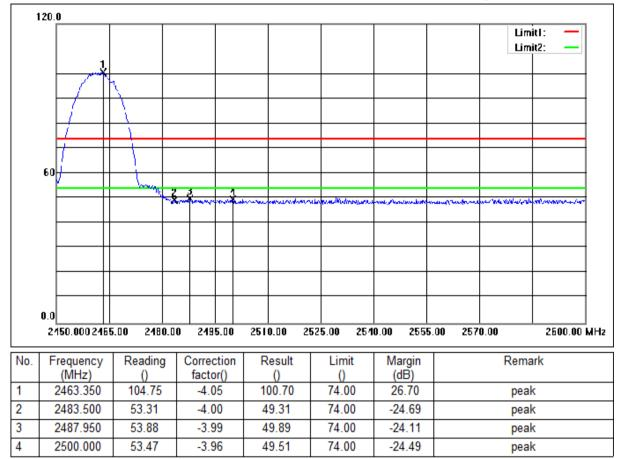
Mode:a; Polarization:Horizontal; Modulation:b; bandwidth:20MHz; Channel:High
