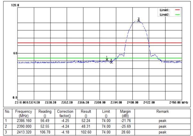
Mode:a; Polarization:Horizontal; Modulation:b; bandwidth:20MHz; Channel:Low
