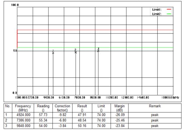
Mode:a; Polarization:Vertical; Modulation:g; bandwidth:20MHz; Channel:High
