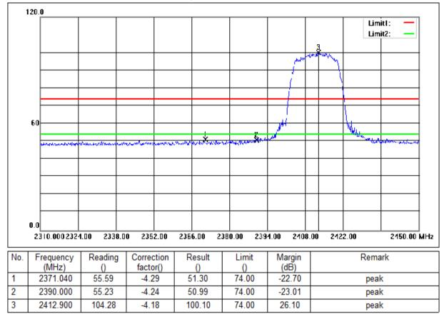
Mode:a; Polarization:Vertical; Modulation:g; bandwidth:20MHz; Channel:Low
