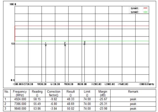
Mode:a; Polarization:Horizontal; Modulation:b; bandwidth:20MHz; Channel:High
