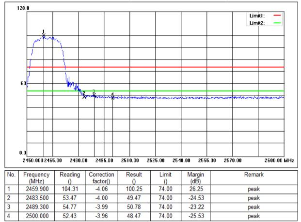
Mode:a; Polarization:Vertical; Modulation:g; bandwidth:20MHz; Channel:High
