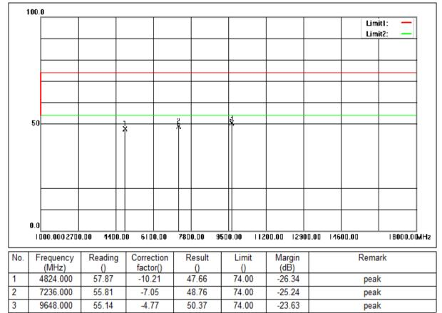
Mode:a; Polarization:Horizontal; Modulation:n; bandwidth:20MHz; Channel:Low
