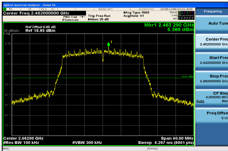
RF Conducted Spurious Emissions_11N20SISO_2462 Ant2
