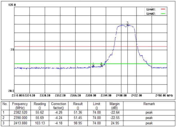
Mode:a; Polarization:Horizontal; Modulation:g; bandwidth:20MHz; Channel:Low
