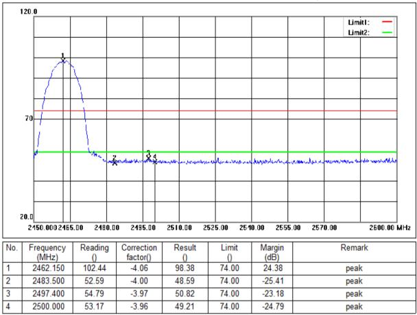
Mode:a; Polarization:Vertical; Modulation:b; bandwidth:20MHz; Channel:High
