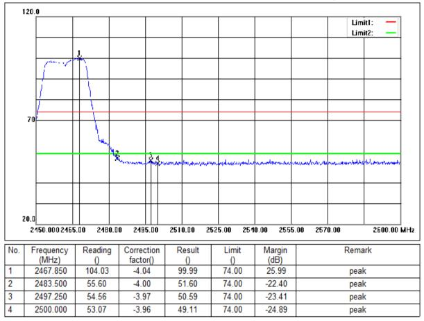
Mode:a; Polarization:Horizontal; Modulation:n; bandwidth:20MHz; Channel:High
