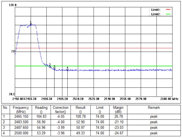
Mode:a; Polarization:Horizontal; Modulation:g; bandwidth:20MHz; Channel:High
