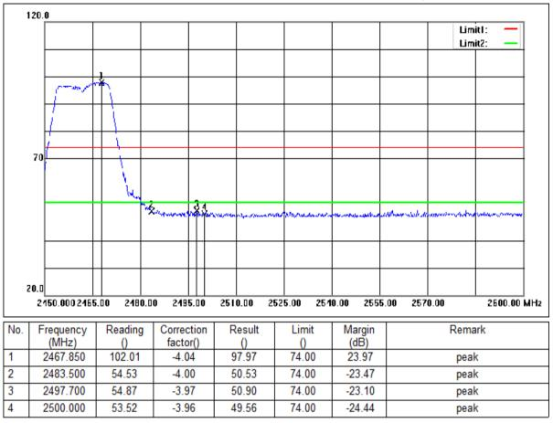
Mode:a; Polarization:Vertical; Modulation:n; bandwidth:20MHz; Channel:High
