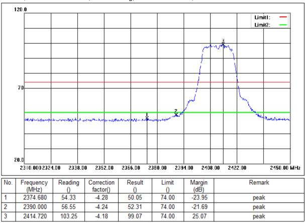
Mode:a; Polarization:Vertical; Modulation:g; bandwidth:20MHz; Channel:Low
