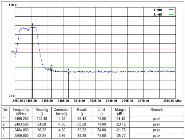
Mode:a; Polarization:Vertical; Modulation:g; bandwidth:20MHz; Channel:High
