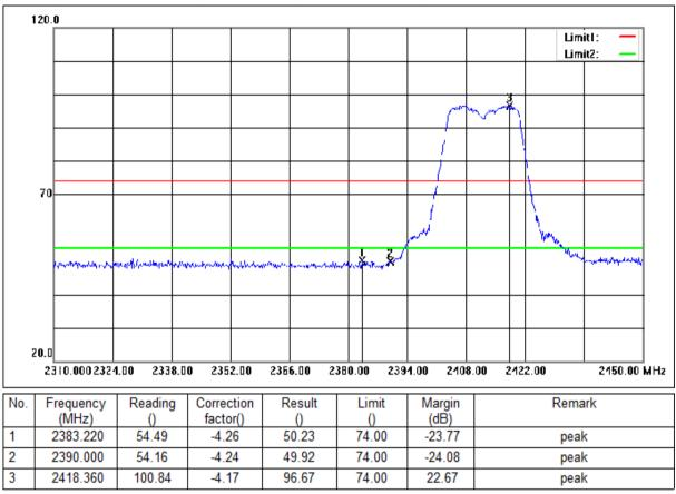
Mode:a; Polarization:Vertical; Modulation:n; bandwidth:20MHz; Channel:Low
