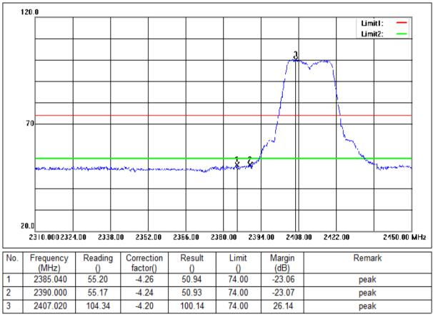
Mode:a; Polarization:Horizontal; Modulation:n; bandwidth:20MHz; Channel:Low
