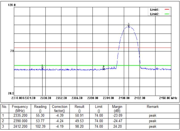
Mode:a; Polarization:Vertical; Modulation:b; bandwidth:20MHz; Channel:Low
