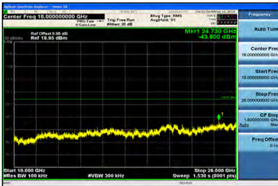
RF Conducted Spurious Emissions_11G_2412
