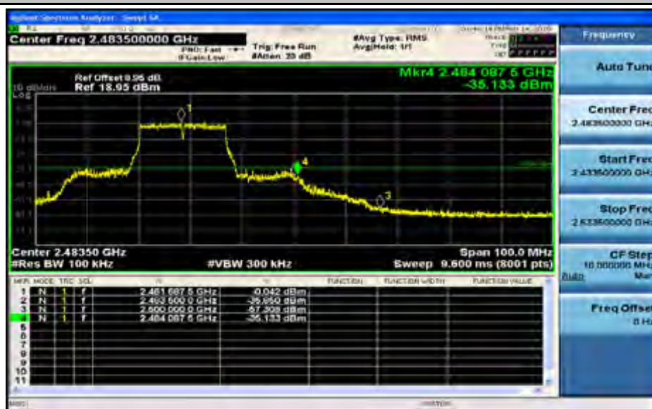
Band-edge for RF Conducted Emissions_11N20SISO_2412_Ant1
