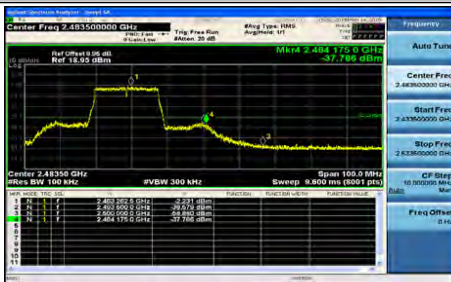
Band-edge for RF Conducted Emissions_11N20SISO_2462_Ant1
