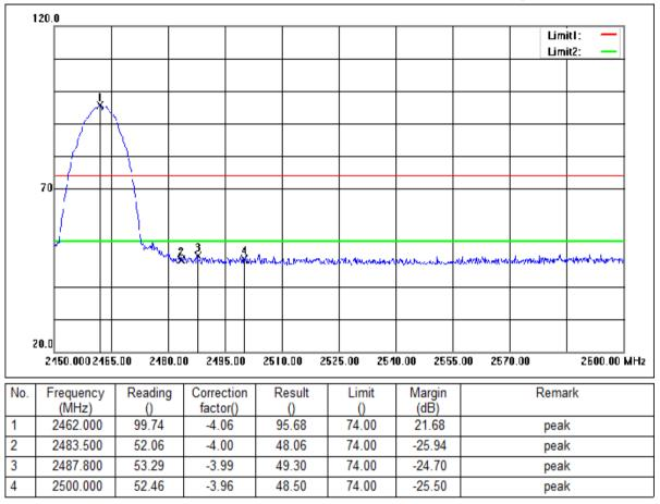
Mode:a; Polarization:Horizontal; Modulation:b; bandwidth:20MHz; Channel:High
