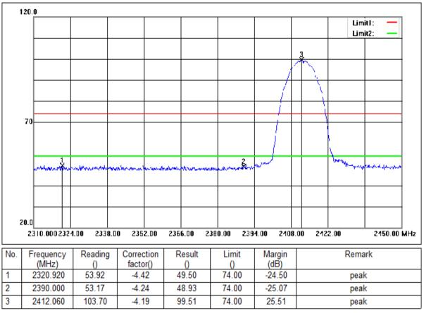
Mode:a; Polarization:Vertical; Modulation:b; bandwidth:20MHz; Channel:Low
