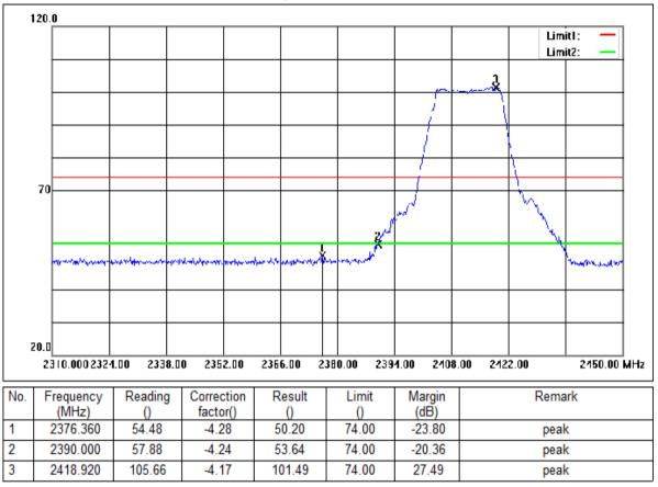
Mode:a; Polarization:Vertical; Modulation:g; bandwidth:20MHz; Channel:Low
