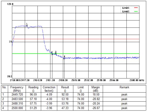
Mode:a; Polarization:Horizontal; Modulation:n; bandwidth:40MHz; Channel:High
