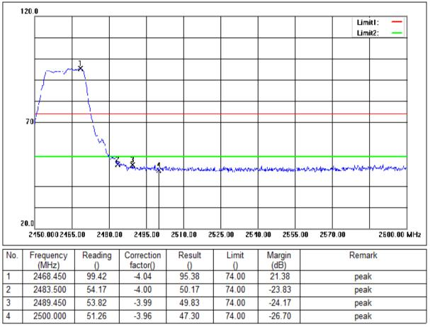
Mode:a; Polarization:Horizontal; Modulation:g; bandwidth:20MHz; Channel:High
