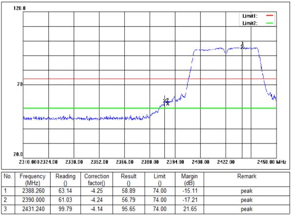
Mode:a; Polarization:Vertical; Modulation:n; bandwidth:40MHz; Channel:Low
