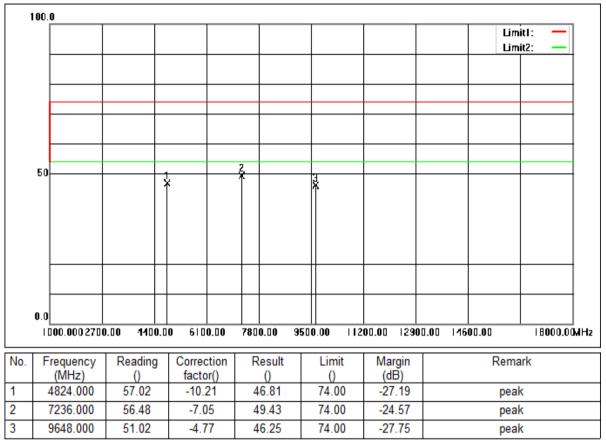
Mode:a; Polarization:Vertical; Modulation:b; bandwidth:20MHz; Channel:Low
