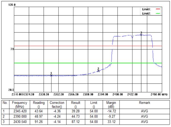
Mode:a; Polarization:Vertical; Modulation:n; bandwidth:40MHz; Channel:Low
