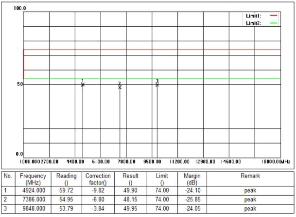
Mode:a; Polarization:Vertical; Modulation:n; bandwidth:20MHz; Channel:High
