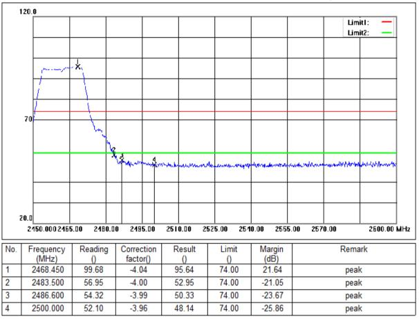
Mode:a; Polarization:Horizontal; Modulation:n; bandwidth:20MHz; Channel:High
