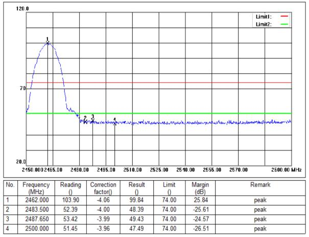
Mode:a; Polarization:Vertical; Modulation:b; bandwidth:20MHz; Channel:High
