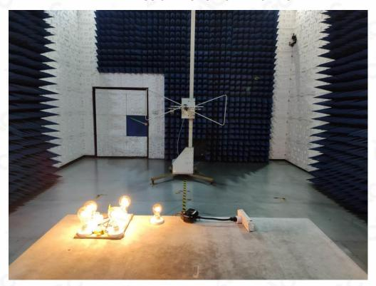
RADIATED EMISSION TEST SETUP ABOVE 1GHz
