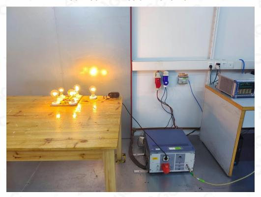
AC POWER LINE CONDUCTED TEST SETUP
