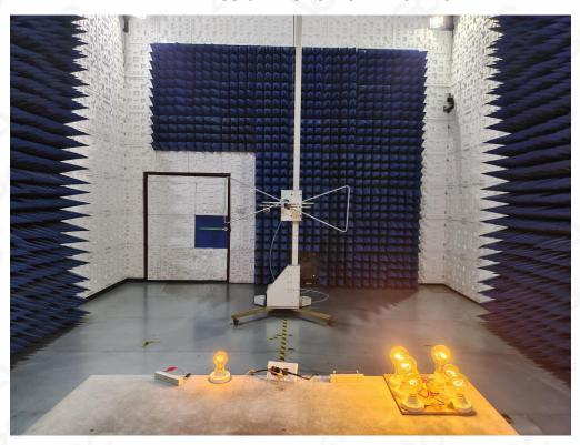
RADIATED EMISSION TEST SETUP ABOVE 1GHz
