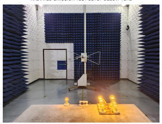
RADIATED EMISSION TEST SETUP ABOVE 1GHz
