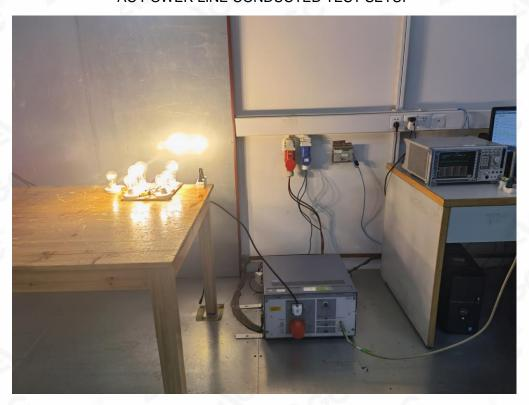
RF CONDUCTED TEST SETUP
