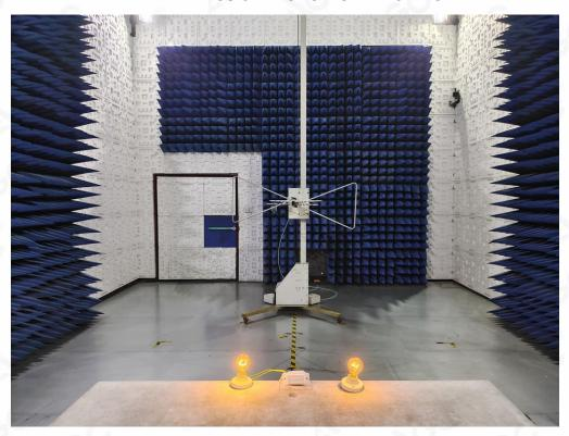
RADIATED EMISSION TEST SETUP ABOVE 1GHz
