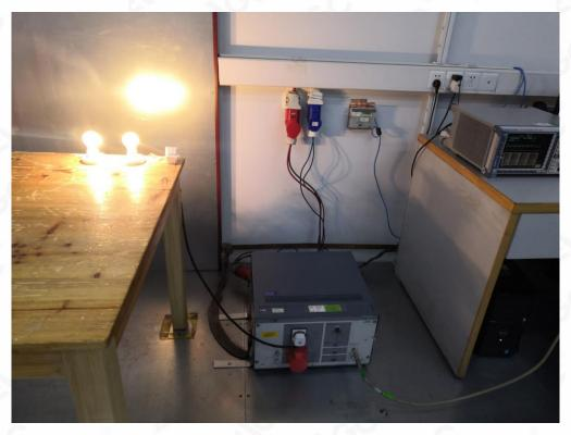
RF CONDUCTED TEST SETUP
