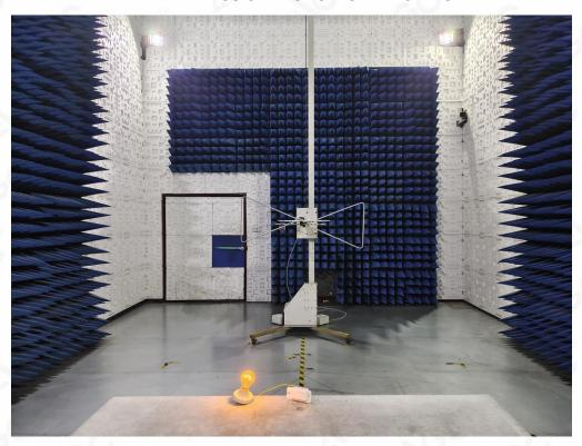
RADIATED EMISSION TEST SETUP ABOVE 1GHz
