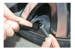
Step 5: Tighten the self-lock nut by special spanner in counter-clockwise direction. Paste warning labels and the installation process is finished.
