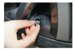
Step 3: Spin the self-lock nut to the inflating valve in the clockwise direction.
