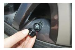
Step 4: Spin the sensor to the inflating valve in the clockwise direction.
