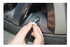
Step 1: Remove the valve sealing cap.
