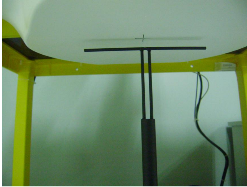
Setup Photo of Dipole Antenna
