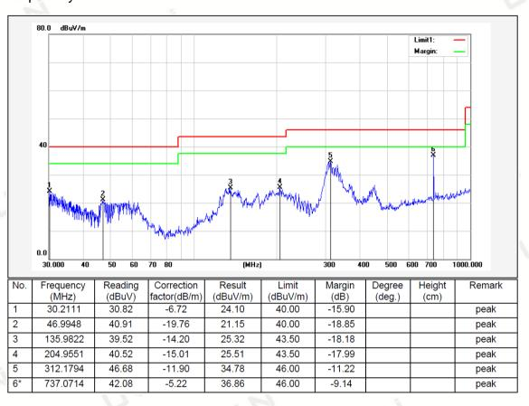
Remark: Absolute Level= Reading Level+ Factor, Margin= Absolute Level – Limit Factor=Ant. Factor + Cable Loss – Pre-amplifi
